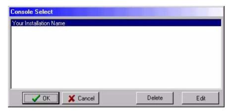
To modify the communication parameters, click on the Edit button on **Screen 13**. Your setup should be similar to the one in **Screen 14**. The *Baud Rate, Port* and *User* information may vary. To setup a new configuration for a different user or a dial up connection, click *Cancel*. From the pull-down menu bar, select *Server* > *Console View* > *New*. **Screen 14** will be displayed without the configuration information. Fill in the data for your new connection.
