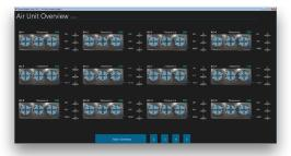
The air unit overview screen will show anywhere from eight to twelve units per screen. This depends on the amount of valves your unit has. Instead of showing piping, we display the valves that are being controlled.
