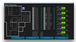
The Main or System overview screen is meant to be a general dashboard showing Air Unit status, fans, temperature and NH3 information, if available, along with System information like king valves, ambient temp and relative humidity.
